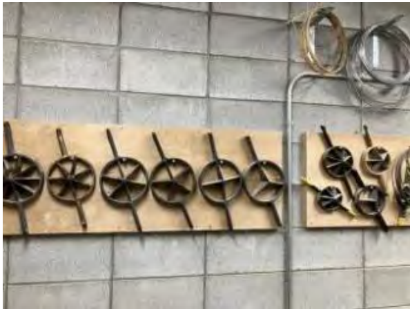
Figure 4. 16 Bamboo craftsman tool for splitting single bamboo pole into different number of pieces possible ranging from three to nine
