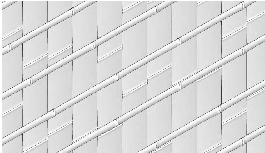
Figure 4. 34 Drawing of flattened bamboo wall, based on Japanese hishigigaki.
